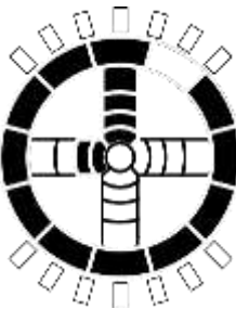
Fig. 14. Display of the dial when the Receiver SNS 1t is located on location line.
